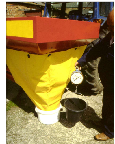
Rate calibration using the manufacturer's rate check kit.
