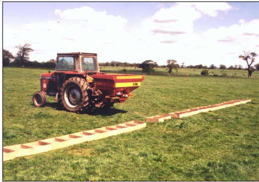
Spread pattern tray testing using a DIY tray test kit (available from IMATS)
